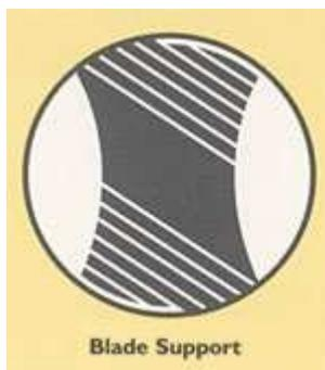
**Reduced Rotational Friction** – By recessing the large radial lands behind the blade, the rotational friction is greatly reduced.
